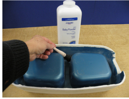
Use a small brush or cotton ball to apply a very thin dusting of talcum powder to the trap.
