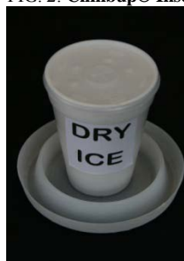
FIG. 2. Climbup® Insect Interceptor with capped cup of dry ice.
